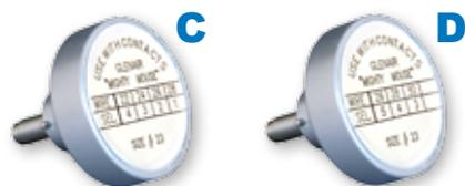
These bayonet-type positioners hold contacts at correct height for crimping with M22520/2 type miniature step adjustable tools, above. Face plate shows correct tool settings.
