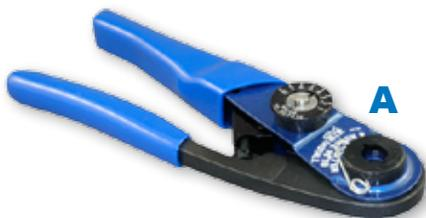
These crimp tools perform precision eight indent crimps for gas tight wire terminations and excellent tensile strength. Adjustment wheel has 8 settings. Ratchet mechanism prevents improper crimps. Use with bayonet type positioners. Check calibration with M22520/3 gages. Length is 6.75 inches, weight is approx. 10 oz.
