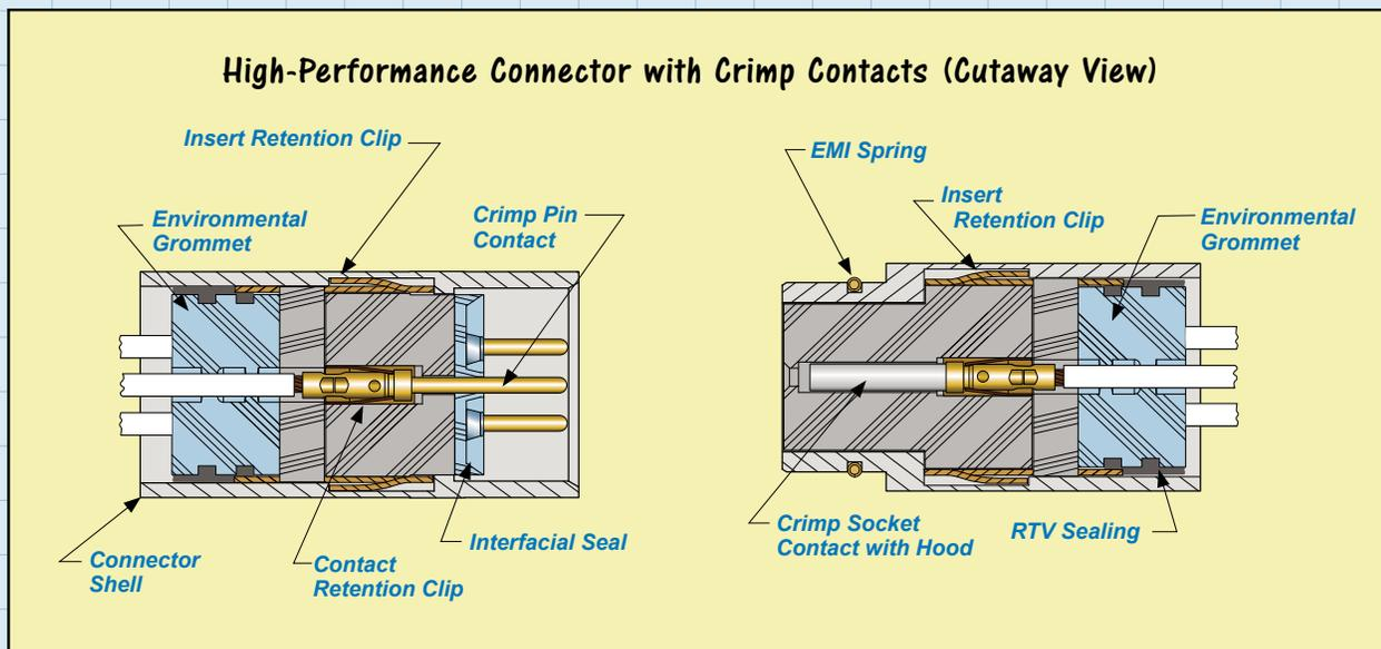
Crimping results in a gas tight connection between the wire and its terminal. Although there are certainly alternatives to crimping, such as ultrasonic welding, resistance welding, insulation displacement technologies and so on, no other available technology delivers the short cycle times, flexibility and low overall cost of crimping—making it the termination technology of choice for most high-performance connector systems.
