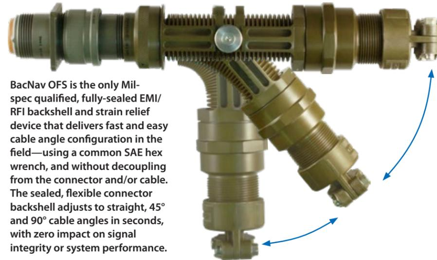
BacNav OFS is the only Mil-spec qualified, fully-sealed EMI/RFI backshell and strain relief device that delivers fast and easy cable angle configuration in the field—using a common SAE hex wrench, and without decoupling from the connector and/or cable. The sealed, flexible connector backshell adjusts to straight, 45° and 90° cable angles in seconds, with zero impact on signal integrity or system performance.
