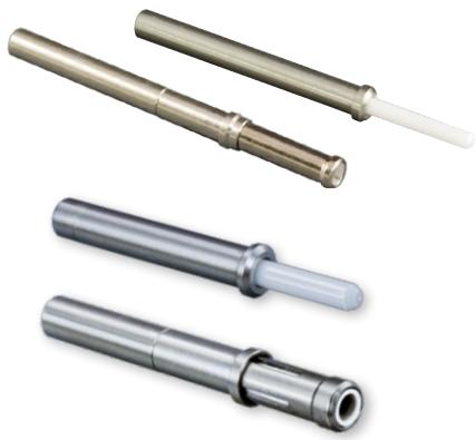
**Single or multimode. Ceramic ferrule. 0.5 dB loss.** Sizes 16 and 20HD fiber optic termini are compatible with Series 806 connectors with sizes 16 and 20HD contact arrangements. These snap-in, rear release termini feature precision ceramic ferrules and alignment sleeves for accurate fiber alignment. Typical insertion loss 0.5 dB. Fits 50/125 and 62.5/125 multimode and 9/125 singlemode fiber.
