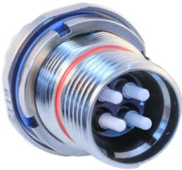
**Micro-Miniature Circular GFR Jam Nut Receptacle.** Supports from two to twelve GFR pin or socket termini with insertion loss performance comparable to industry-standard MIL-PRF-29504. Precision-machined with O-ring environmental seal. Back-end threads and teeth accept Glenair Mighty Mouse accessories. Available in aluminum and stainless steel. Termini sold separately. Supports single- and dual-O-ring termini.
