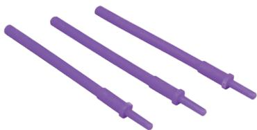
Dummy sealing plugs maintain environmental sealing in empty rear-release crimp connector cavities. Made of chemical-resistant thermoplastic, these dummy contacts are available in sizes 16 and 20HD. Sealing plug tail protrudes from grommet to facilitate removal with standard extraction tools. Rated for +200 °C continuous operating temperature, these sealing plugs save weight compared to installing both an unused contact and a grommet sealing plug.
