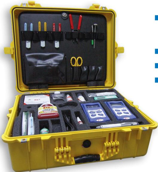
Our termination kit allows field technicians the convenience of on-site optical fiber termination. Each kit contains jacket strippers, polishing tools, hand tools, light source, power meter and microscope as well as a full complement of consumables including epoxy, polishing media, swabs and adhesives.
