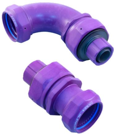
Series 377-014 supports both PEEK as well as Glenair Series 74 Teflon type convoluted tubing with either band attachment or lamp-thread (nut) attachment. All styles equipped with fiber alignment grommet matched to shell size.
