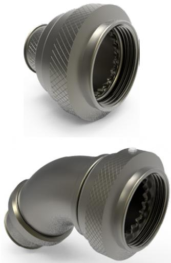
Series 44 environmental backshells with straight, swept 45° and 90° profiles are ideal for combo copper /fiber insert arrangements where EMI/RFI shielding and environmental sealing are needed. Anti-decoupling device for improved vibration resistance and detents to allow for axial positioning of backshell for improved cable routing.
