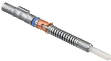
The Glenair High Density Fiber Optic Connection System is designed for applications that require reduced size and weight as well as outstanding optical and environmental performance. The System offers insertion loss values less than 0.5dB (typical loss for Glenair termini is 0.3 dB). Dense cavity spacing is achieved with an innovative front release terminus design and accommodation for M85045/16 cable. The 181-047 version is equipped with a single keying feature for APC polish.
