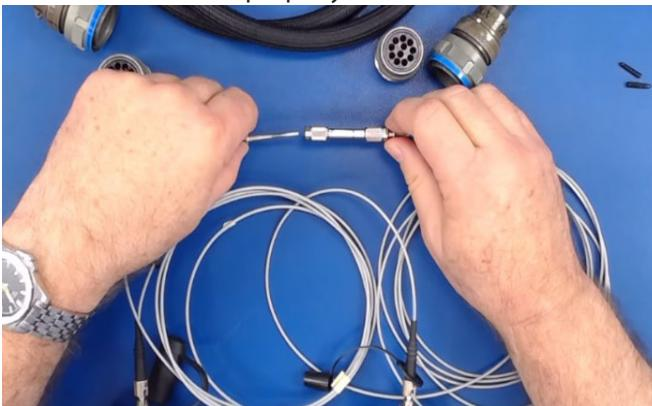
3. Zero out test probe adapters by pressing and holding the button labeled dB/dBm. Readout is in dB.
