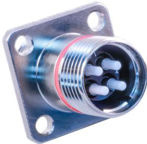
**Micro-Miniature Circular GFR Wall Mount Receptacle.** Supports from two to twelve GFR pin or socket termini with insertion loss performance comparable to industry-standard MIL-PRF-29504. Precision-machined with O-ring environmental seal. Back-end threads and teeth accept Glenair Mighty Mouse accessories. Available in aluminum and stainless steel. Termini sold separately. Supports single- and dual-O-ring termini.
