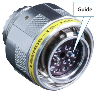
Guide pins facilitate repeatable optical performance by ensuring alignment between mating cavities. Threaded-coupling connectors without guide pins can "sweep" relative to each other when torqued. Misaligned cavities will force the split ceramic alignment sleeve to work harder to bring mating termini into alignment. Stressed alignment sleeves can expand (and possibly break), resulting in high optical loss.
