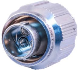
**Micro-Miniature Circular GFR Plug.** Supports from two to twelve GFR pin or socket termini with insertion loss performance comparable to industry-standard MIL-PRF-29504. Precision-machined with O-ring environmental peripheral seal. Back-end threads and teeth accept Glenair Mighty Mouse accessories. Available in aluminum and stainless steel. Termini sold separately. Supports single- and dual-O-ring termini.
