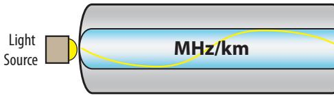
**Bandwidth Limited Operation** The condition prevailing when the system bandwidth, rather than the amplitude of the signal, limits performance. The condition is reached when modal dispersion distorts the shape of the waveform beyond specified limits.
