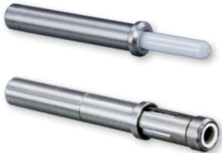
Single or multi mode. Ceramic ferrule. 0.5 dB loss. Size 16 fiber optic termini are compatible with Series 806 connectors with size 16 contact arrangements. These snap-in, rear release termini feature precision ceramic ferrules for accurate fiber alignment. Typical insertion loss 0.5 dB. Fits 50/125 and 62.5/125 multi mode and 9/125 single mode fiber.
