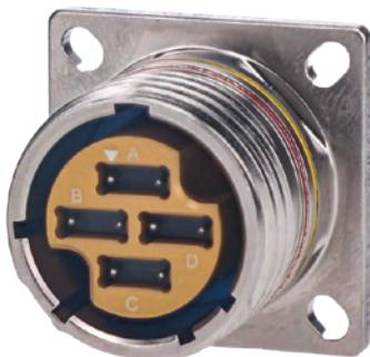
**Glenair SOSA-Compliant VITA 87** is a High-Density Mil-Aero Grade MT Fiber Optic Connector. Utilizes the tried and true MIL-DTL-38999 Series III connector packaging for use with Standard and Prizm MT Ferrules. Available in 3 shell sizes, starting as small as a Shell Size 11 with 1 MT to a Shell Size 15 with 4 MT's.
