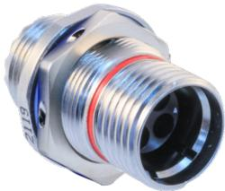
**Micro-Miniature Circular GFR Jam Nut Receptacle with Safety Wire Holes.** Supports from two to twelve GFR pin or socket termini with insertion loss performance comparable to industry-standard MIL-PRF-29504. Precision-machined with O-ring environmental seal. Back-end threads and teeth accept Glenair Mighty Mouse accessories. Available in aluminum and stainless steel. Termini sold separately. Supports single- and dual-O-ring termini.
