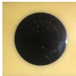
Reinforced solder joint with potting
