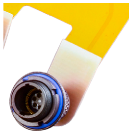
Stiffeners at critical assembly points
