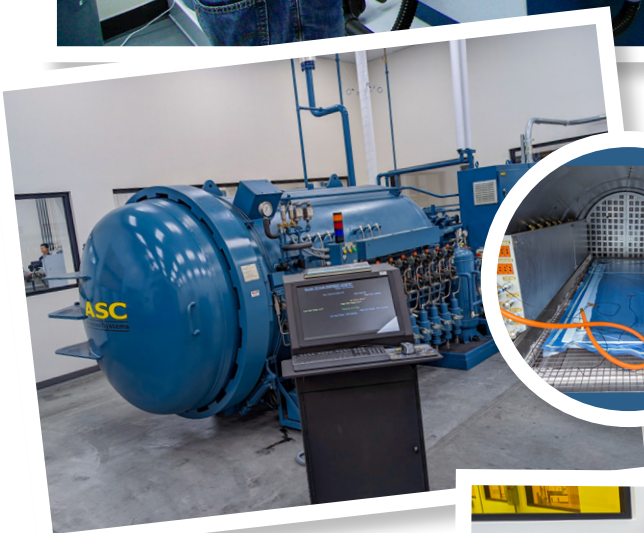
ASC Autoclave enabling continuous lamination up to 96 inches
