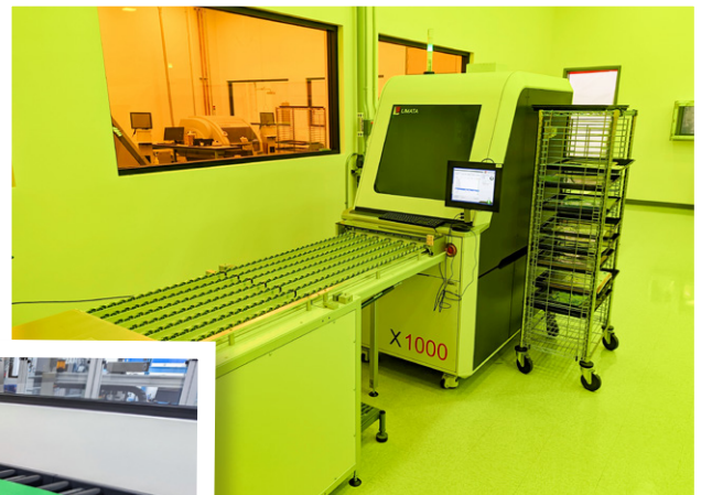
Limata laser direct imaging system for extended length flex circuits
