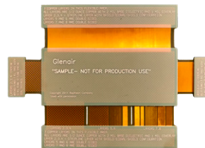
Complimentary quick-turn mockups produced by by Glenair: 28-layer rigid flex, and 12-layer multibranch rigid flex
