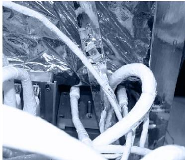
**Detail of the Atmospheric Infrared Sounder (AIRS) with Glenair Micro-D Cables and Connectors**
