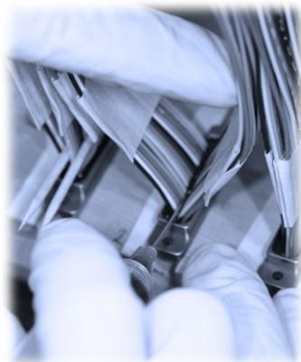
**Potting a Micro-D with Epoxy-Filled Syringe**
