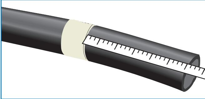
**B)** Score insulation lengthwise along the entire section of insulation to be removed.
