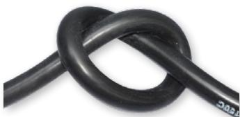
TurboFlex bend radius (Duralelectric jacketing) is 3X the outer diameter
