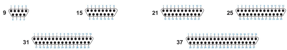
Mating face of pin connector. Socket connector contact numbers are reversed.
