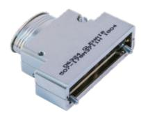
**Split Backshell With Elliptical Cable Entry** provides added room for larger wire bundles. Terminate cable shields with Band-Master ATS® Micro Bands. This backshell features floating male screwlocks which allow full mating of the connector before the screws are fastened.
