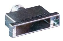
**Save Weight and Eliminate Corrosion Damage** with composite Micro-D backshells. These round cable entry backshells are injection-molded with high strength Ultem 2300 fiberglass-reinforced thermoplastic.
