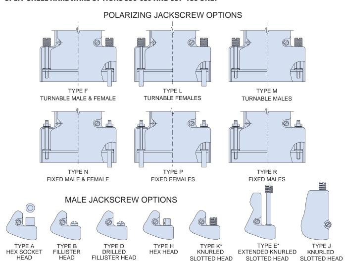
Unless otherwise noted, all jackscrews have 4-40 UNC-2A threads to mate with M24308/26 female screwlocks or 559-001 mounting kits. (Not applicable for cable-to-cable applications.)
