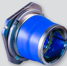
**Float mount:** allows for a modicum of coplanar movement of the receptacle during rack-and-panel and other blind mate applications, preventing both contact and shell damage.
