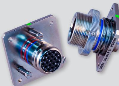
**Assisted separation force:** Glenair supplies two styles of spring-loaded blind-mate connectors. **Adjustable kick-off styles** feature spring-loaded posts on the plug and an adjustment ring on the receptacle used to calibrate separation force. The second style uses wave springs on the shell body.
