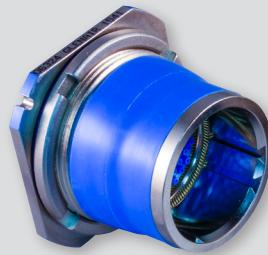
**EMI shielding:** Glenair incorporates ground springs in receptacle connectors as well as grounding fingers in special coupling nut-equipped plugs (253-018-G6 feed-thru shown) to optimize 360° shell-to-shell continuity.
