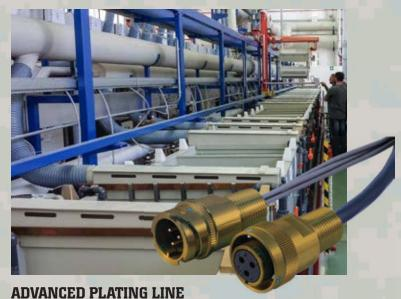
Capabilities include VG95328-qualified Marine Bronze and "Code J" Tin-Zinc plating—VG95211 and VG95212 qualified cadmium alternative for corrosion-resistant interconnects.
