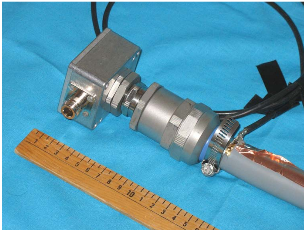
Figure 3. Measurement End of Glenair M24758 Conduit, with IEC 600096-1, Amendment 2 Test Apparatus Installed.
