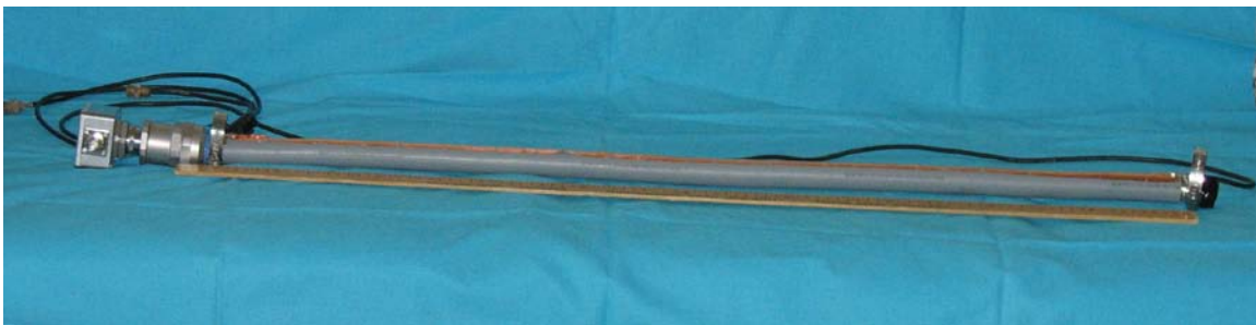
Figure 1. Glenair M24758 Conduit Assembly, with IEC 600096-1, Amendment 2 Test Apparatus Installed. A 1-m scale is included.
