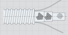
Glenair can supply lengths of polymer-core tubing with pre-installed mule tape lanyards to make on-site installation of wire bundles through tubing easier. Polymer tubing can also be supplied with stress members in Nomex, Kevlar, or CRES stainless steel to provide conduit with enhanced pull strength and stress resistance.
