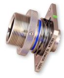
Misalignment accommodation: Radial, axial, and angular misalignment in blind-mate applications is resolved in the receptacle design with mechanical float mounting and integral wave form springs.
