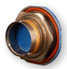
EMI shielding: Glenair blind-mate circulars are available with auxiliary ground springs on receptacles, and ground fingers on plugs (shown), to optimize 360° shell-to-shell continuity.
