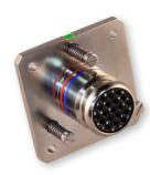
Assisted separation: Springloaded kick-off posts are designed to overcome contact separation force (normal force) with adjustable flange-mounted springs. Separation force may be calibrated IAW application requirements and insert arrangement.
