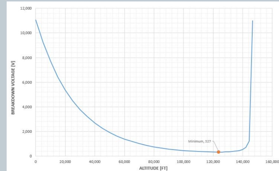
When an interconnect is used in applications at high altitudes, ambient pressure is reduced. Unless the insulation system is hermetically sealed, the pressure of the insulating air is reduced as well. As the insulating air loses pressure, it also loses strength, and weakens the overall insulation system. Therefore, interconnect products perform best at sea-level, and must be derated for high-altitude applications.
