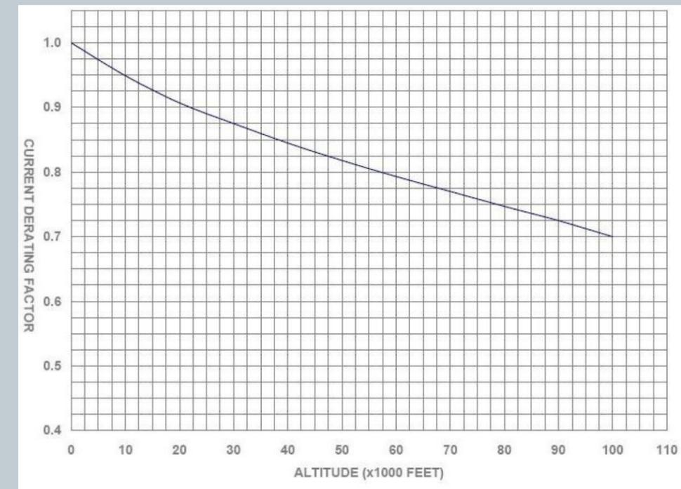
Source: Figure 5, “Altitude Derating Curve” SAE AS50881; 2015
