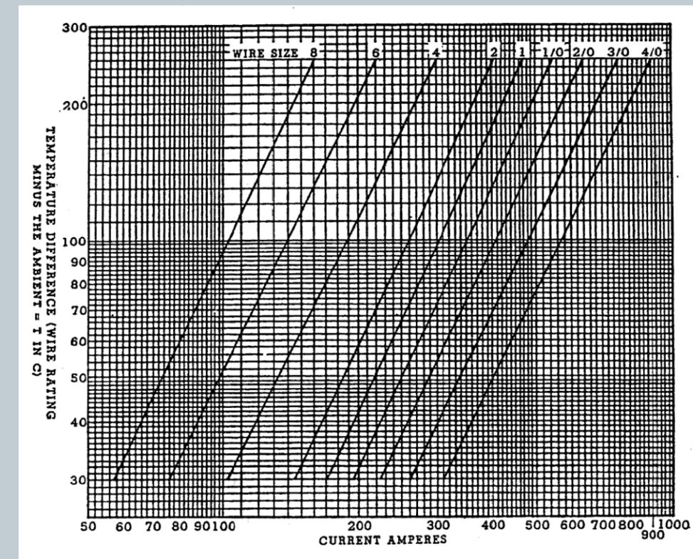
Source: Figure 3, "Single Copper Wire in Free Air," SAE AS50881; 2015
