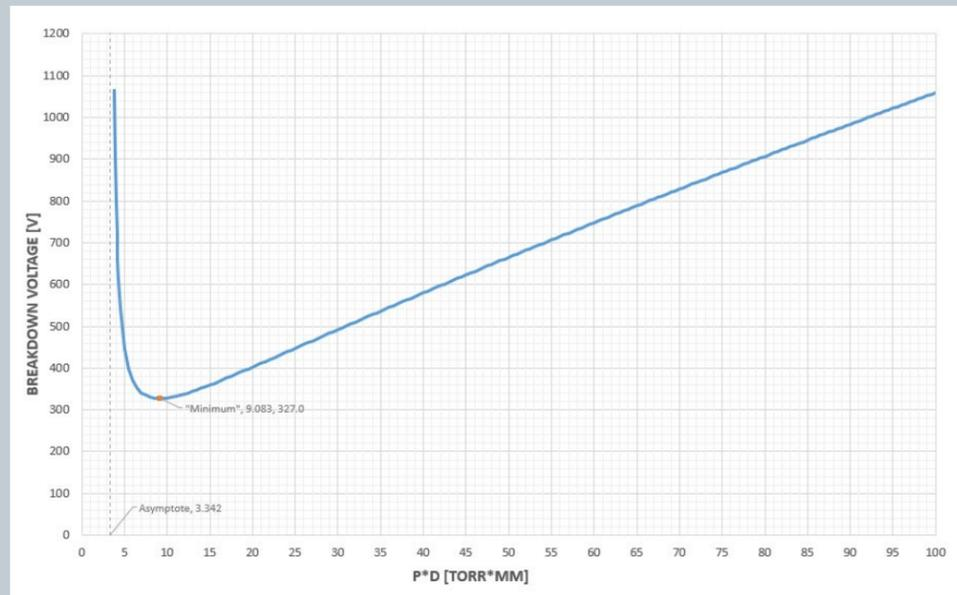
As shown in Figure 1, when pressure is reduced (“P”), the breakdown voltage (“V”) is also reduced (assuming constant air gap, “D”). However, this is only true until “Paschen’s Minimum” is reached (typically ~327 VDC). At pressures below Paschen’s Minimum, the air starts to behave more like a vacuum and strength is increased (vacuums are nearly perfect insulators).
