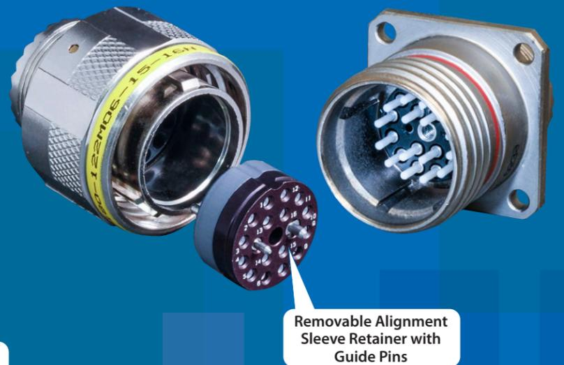
Guide Pins facilitate repeatable optical performance by ensuring alignment between mating cavities. Threaded-coupling connectors without guide pins can "sweep" relative to each other when torqued. Misaligned cavities will force the split ceramic alignment sleeve to work harder to bring mating termini into alignment. Stressed alignment sleeves can expand (and possibly break), resulting in high optical loss.
