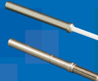
Single or multimode. Ceramic ferrule. 0.5 dB loss. Size 20HD fiber optic termini are compatible with Series 806 connectors with size 20HD contact arrangements. These snap-in, rear release termini feature precision ceramic ferrules and alignment sleeves for accurate fiber alignment. Typical insertion loss 0.5 dB. Fits 50/125 and 62.5/125 multimode and 9/125 singlemode fiber.
