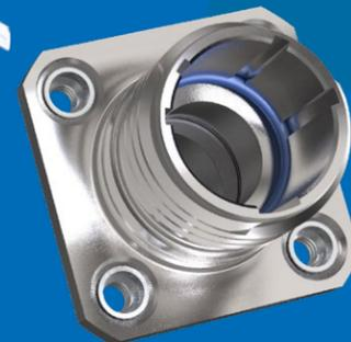
The O-ring peripheral seal not only provides an excellent moisture seal, but also a mechanical and electrical benefit. Because the O-ring displaces radially, it allows full metal-to-metal bottoming without the use of tightening tools. This feature, combined with the shallow ramp threads, results in secure, vibration-resistant coupling by hand, no tool required. Metal-to-metal bottoming is essential for long-term mechanical survivability, EMI, and shell-to-shell conductivity.
