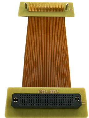
HD Stacker board-to-board connector/flex mockup
