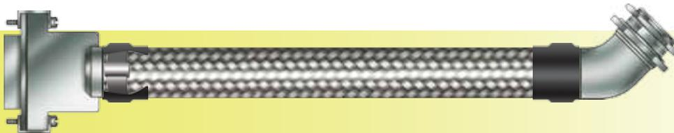
**T**his cutaway view shows band termination of conduit overbraid under the protective shrink sleeves that are supplied with all braided assemblies. The BAND-IT® band terminates the braid at the connector end for 360° EMI/RFI shielding.
