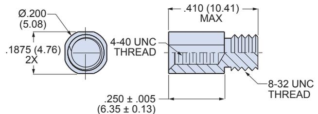
Style "P" jackpost has #8-32 thread for installation into panel mount HiPer-D® connectors with corresponding #8-32 tapped flange. 300 series stainless steel, passivated. One kit consists of (2) jackposts. Install with threadlocking compound. Mates with all standard #4-40 male screw locks and jackscrews.
