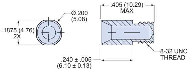
Style "B" guide bushing for blind mate applications has #8-32 thread for installation into panel mount HiPer-D® connectors with corresponding #8-32 tapped flange. 300 series stainless steel, passivated. One kit consists of (2) bushings. Install with threadlocking compound. Mates with style "G" guide pin 289-014-G.
