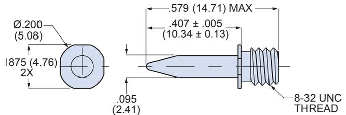
Style "G" guide pin for blind mate applications has #8-32 thread for installation into panel mount HiPer-D® connectors with corresponding #8-32 tapped flange. 300 series stainless steel, passivated. One kit consists of (2) guide pins. Install with threadlocking compound. Mates with style "B" guide bushing 289-014-B.
