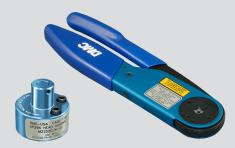
809-127 (M22520/4-01) crimper for use with size #16 coax Series 806 contacts. Requires positioner, ordered separately. These crimp tools perform precision eight indent crimps for wire terminations and excellent tensile strength. Ratchet mechanism prevents improper crimps. Use with bayonet-type positioners. Length is 9.75 inches, weight is 15 oz.
