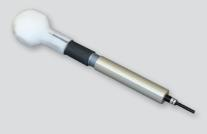
Check for properly seated contacts with this spring-loaded tester. Apply the tool tip to the mating end of a contact. Push on the handle until the spring compresses to the recommended force. A visual indicator shows full compression. The contact is properly retained if it is not displaced. Pin tips are used with pin contacts. Socket tips are used with socket contacts. Complete kit options available, or order the tips and handles separately.
