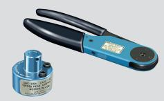
809-133 (M22520/31-01) crimper for use with size #12 Series 806 coax contacts. Requires positioner, ordered separately. These crimp tools perform precision eight indent crimps for wire terminations and excellent tensile strength. Adjustment wheel has 8 settings for wire being used. Ratchet mechanism prevents improper crimps. Use with bayonet-type positioners. Length is 9.75 inches, weight is 15 oz.
