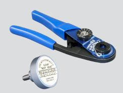
809-015 (M22520/2-01) crimper for use with size #20HD and #22HD signal contacts and #8, #12, #16 co-axial and tri-axial Series 806 contacts. Requires positioner, sold separately. These crimp tools perform precision eight indent crimps for wire terminations and excellent tensile strength. Adjustment wheel has 8 settings. Ratchet mechanism prevents improper crimps. Use with bayonet-type positioners. Length is 6.75 inches, weight is approx. 10 oz.
