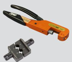
Standard 809-129 (M22520/5-01) crimper. Use with size #8 twinax and quadrax Series 806 RF contacts. Requires hex-die, ordered separately. These crimp tools attach contact body to cable. Length is 11 inches, weight is approx. 1.476 lbs. For use with interchangeable coax hex-dies. Dies snap in frame of M22520/5-01 and are held in frame by internal spring clips.
