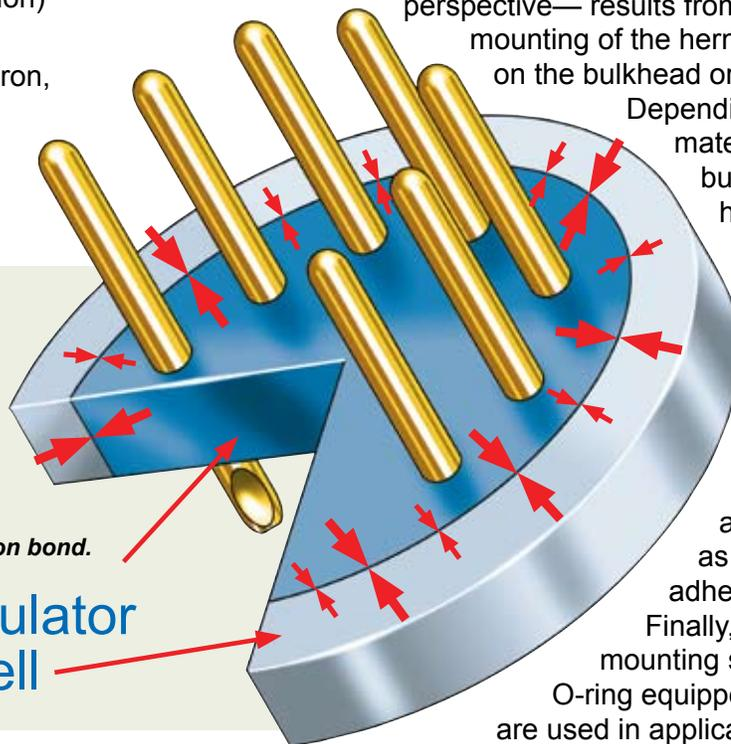
Kovar is a low-expansion metal with a coefficient of expansion rating matched to the glass material that forms the hermetic seal.
