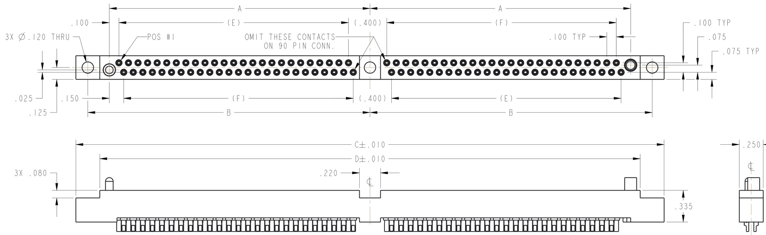
FIGURE 2. RECEPTACLE CONNECTOR, SOLDER CUP SOCKET CONTACTS (2 BAY)
