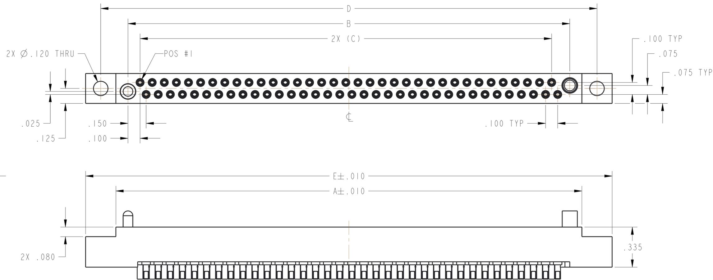
FIGURE 1. RECEPTACLE CONNECTOR, SOLDER CUP SOCKET CONTACTS (1 BAY)
