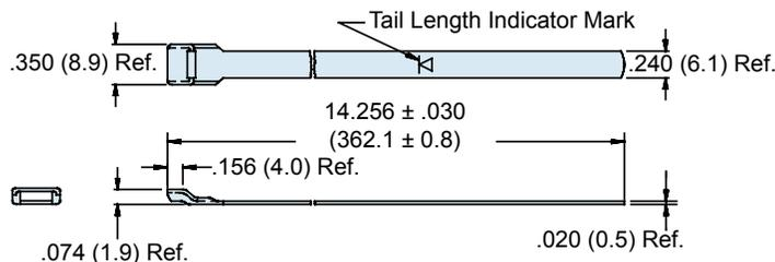
**The M85049/128-3 and -4 Standard Band** is precision constructed of 300 Series SST/ Passivate and designed for use with the Glenair 600-058 (QPL'd) hand banding tool, double-wrapped bands will accommodate diameters up to approximately 1.8 inches (45.7). Bands may be ordered flat (M85049/128-3) or precoiled (M85049/128-4). Bands come bagged and tagged in quantities from 1 to 100.
