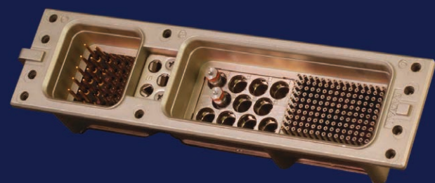
ARINC 600 rack-and-panel connector with drop-in sie #8 optoelectronic contacts for use in a commercial aircraft data server application.
