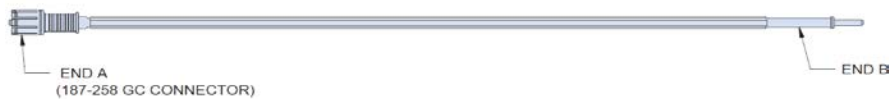
FIGURE 5 Fiber Optic Jumper Cable Assembly (see separate Glenair sales drawing FA02454 for details)
