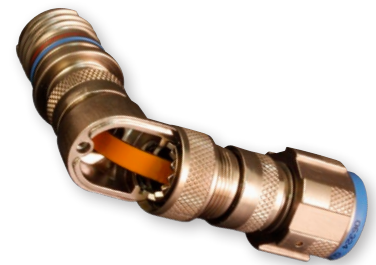
High-shock matched-impedance Mighty Mouse assembly with flex circuit
