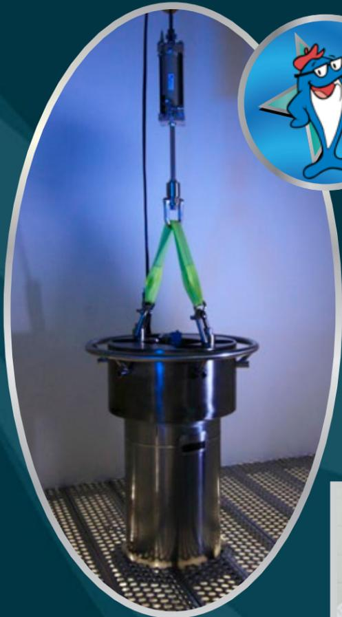
**2. Large cable and subassembly pressure test bunker**
