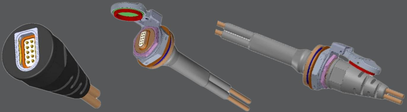
Overmolded environmental plug. CAD drawing shows polarized shape of mating interface as well as internal sealing and retention spring.
