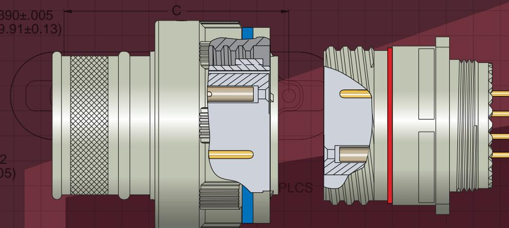
Circular connector coupling technology: the ubiquitous MIL-DTL-38999 Series III circular features one of the most popular connector coupling designs, the triple-start stub ACME thread. In addition to fast and reliable mating, this threaded coupling design has the advantage of a ratcheting anti-decoupling mechanism, receptacle striping indicating full mating, and metal-to-metal bottoming between the mating pairs for reduced electrical resistance.
