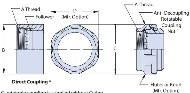
Note: Code G, rotatable coupling is supplied without O-ring.
