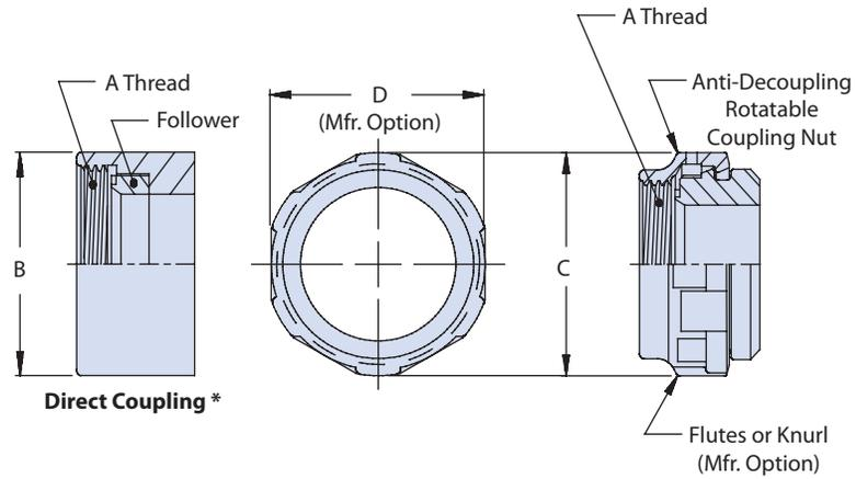
Note: Code A, rotatable coupling supplied without O-ring.
