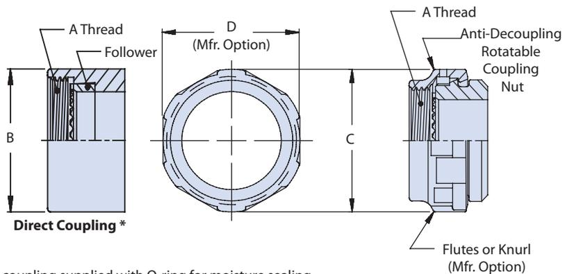
Note: Direct coupling supplied with O-ring for moisture sealing.
