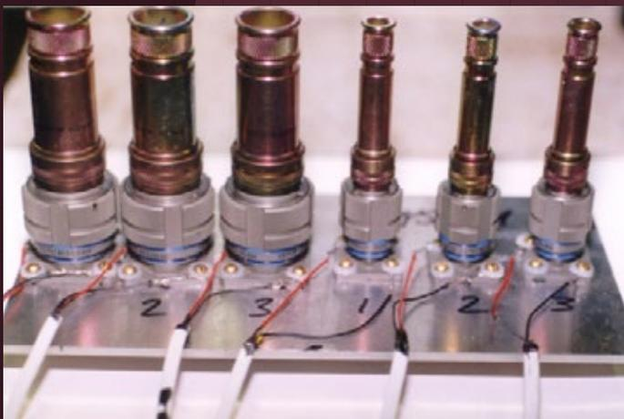
Connector testing is designed to simulate a lifetime of use over a short period of time. Environmental, mechanical and electrical tests are conducted to measure both the reliability of the connector and the system. The number-one criterion of reliability is a change in contact resistance.
