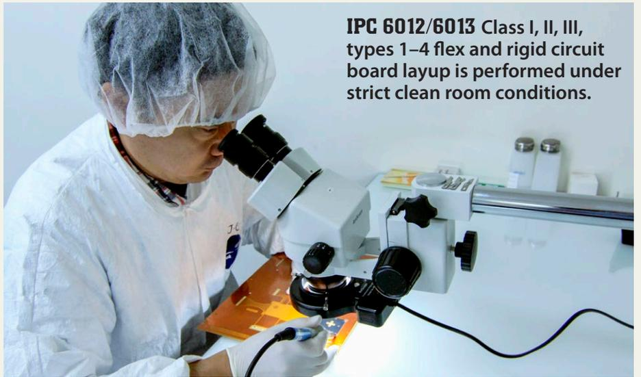
**IPC 6012/6013 Class I, II, III, types 1-4 flex and rigid circuit board layout** is performed under strict clean room conditions.
