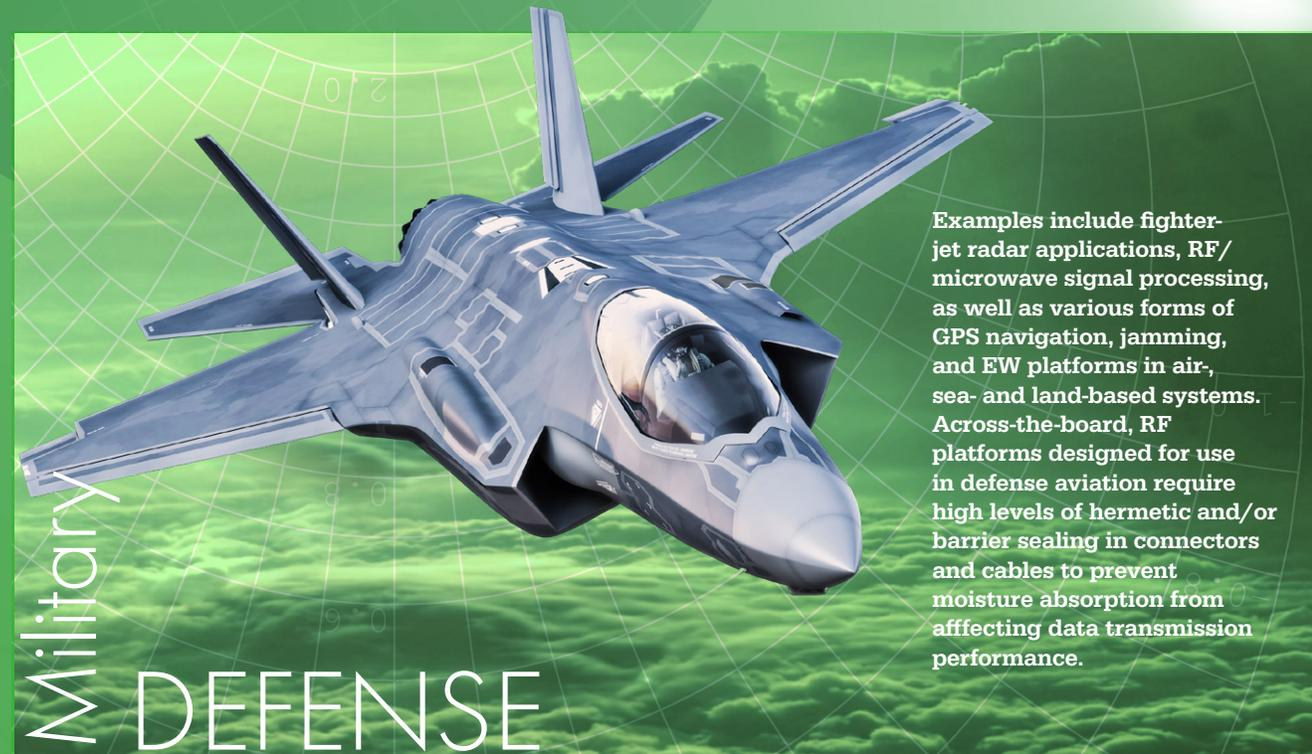
Examples include fighter-jet radar applications, RF/microwave signal processing, as well as various forms of GPS navigation, jamming, and EW platforms in air-, sea- and land-based systems. Across-the-board, RF platforms designed for use in defense aviation require high levels of hermetic and/or barrier sealing in connectors and cables to prevent moisture absorption from affecting data transmission performance.
