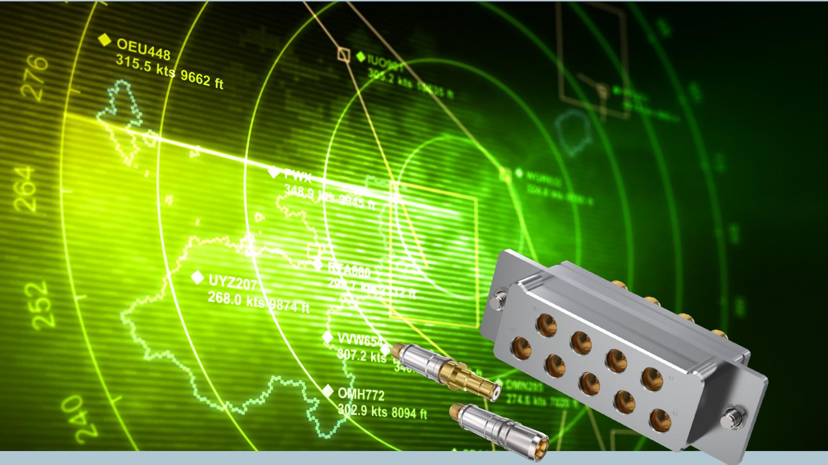
The Glenair Series 795 is a multiport aerospace-grade coax connector designed for use with snap-in and removable size #8, #12, and #16 coax contacts from DC to 65 GHz frequency. Environmentally protected and EMI shielded for harsh application environments.
