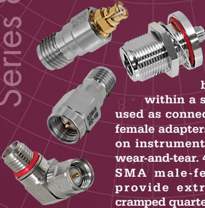
Precision - grade Series 852 RF Adapters are used to connect between series or within a series. Frequently used as connector savers, male-female adapters protect RF jacks on instruments from excessive wear-and-tear. 45° and 90° angled SMA male-female adapters provide extra clearance in cramped quarters.
