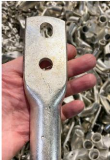
**Tin-plated copper** material is commonly used in most aerospace applications, and combines the excellent conductivity of
