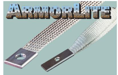
**ArmorLite™:** Uniquely available from Glenair, ArmorLite is an additional material choice for use in grounding and bonding. ArmorLite is a nickel- or silver-clad stainless steel micro-filament material that saves significant weight compared to standard QQ-B-575 materials such as soft-drawn silver- and tin-plated copper.
