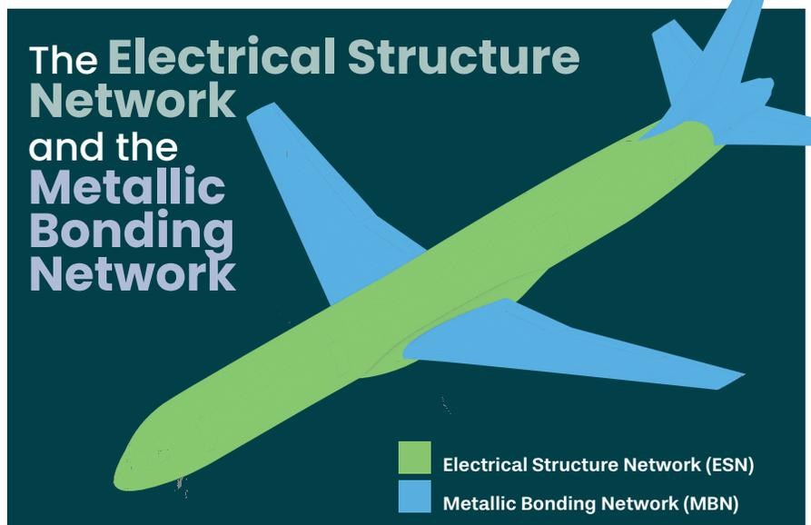
Modern aircraft are equipped with two distinct but interconnected systems, the “Electrical Structure Network” and “Metallic Bonding Network”
