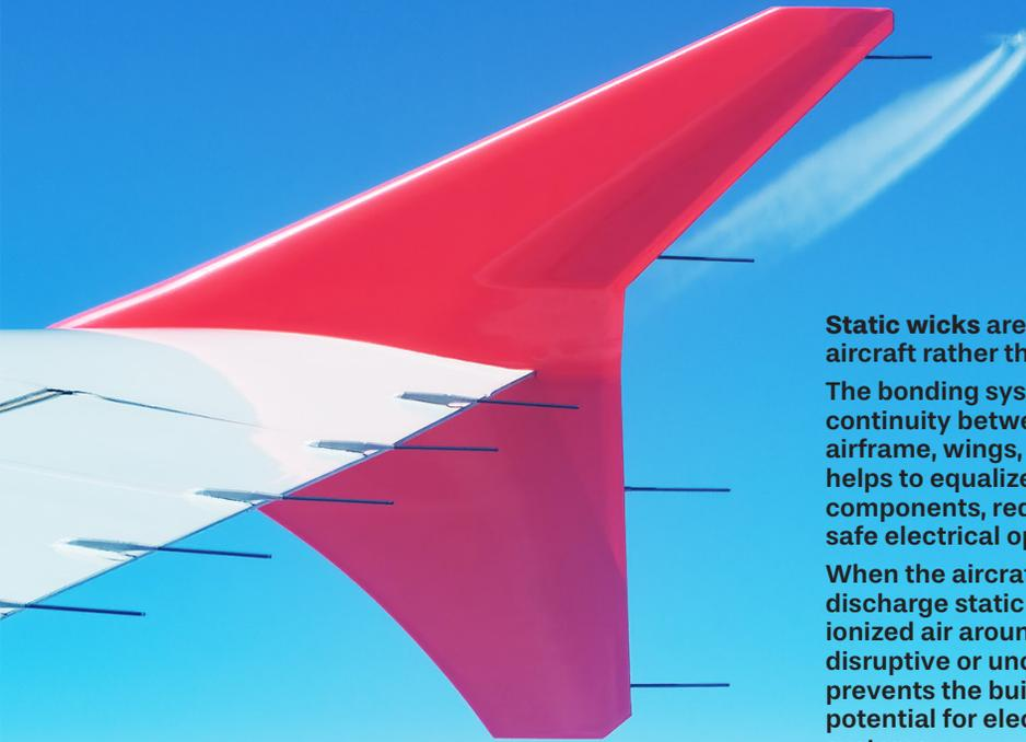
**Static wicks** are considered a part of the "bonding" system on an aircraft rather than the "grounding" system.
