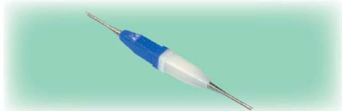
*New for 2006: a top-notch "Mighty Mouse" contact insertion and removal tool designed for reliable performance with all supported wire sizes.*
