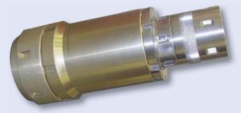
Special strain-relief backshell invented by Glenair for use on the French TGV rail system. This backshell design resolved complex intercar vibration and shock prolems which resulted in destructive cable damage.
