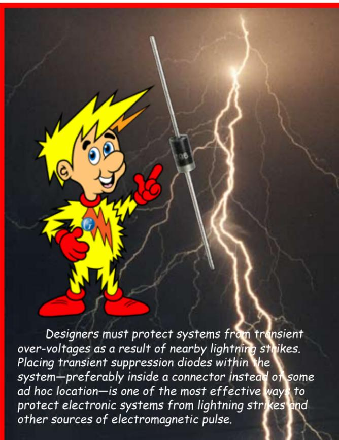
Designers must protect systems from transient over-voltages as a result of nearby lightning strikes. Placing transient suppression diodes within the system—preferably inside a connector instead of some ad hoc location—is one of the most effective ways to protect electronic systems from lightning strikes and other sources of electromagnetic pulse.
