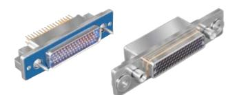
Micro-Crimp panel mount connectors are ideal for module-to-chassis packaging. Stainless steel guide pins assure connector alignment for blind mate applications. Float bushings are also available.
