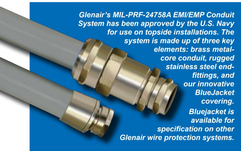
*Glenair's MIL-PRF-24758A EMI/EMP Conduit System has been approved by the U.S. Navy for use on topside installations. The system is made up of three key elements: brass metal-core conduit, rugged stainless steel end-fittings, and our innovative BlueJacket covering. Bluejacket is available for specification on other Glenair wire protection systems.*
