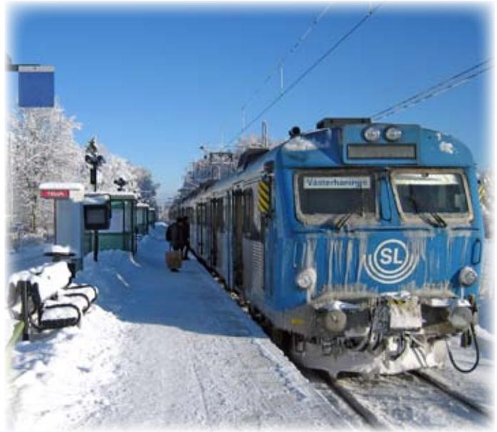
***The “pilot” protects the locomotive and its engineers by deflecting obstacles away from the train. Interconnect wiring behind the pilot sees some mighty rough duty.***
