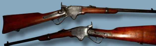
7. Developed during the American Civil War, the **Spencer Carbine was the first true repeating rifle**, capable of firing up to 20 rounds a minute. The 1865 Spencer .50 caliber, and later weapons modeled after it, precipitated the fielding of smaller units of soldiers deployed in more agile and flexible formations. The increased volume of fire and deadly accuracy of the Spencer put an end to the 19th Century tactics of massed troops fighting in formation.
