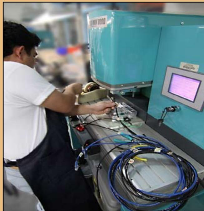
**State-of-the art equipment and production systems add speed and reliability to the overmolding process. In this photo, a skilled technician is prepping a Series 80 Mighty Mouse cable for overmolding.**
