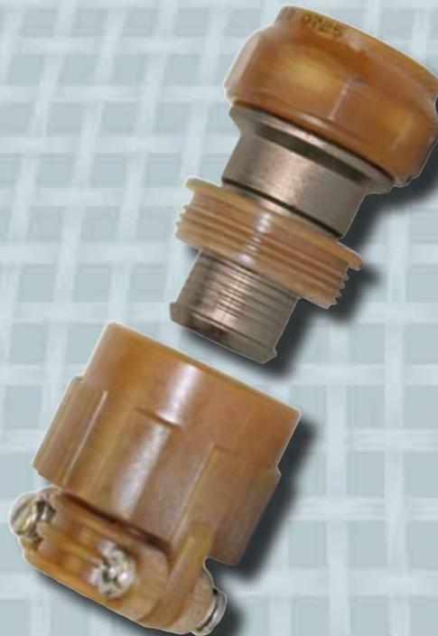
*Thermoplastic connector components, such as this Band-in-a-Can Backshell, may be selectively plated with conductive material. This strategy enables users to enjoy the weight saving and durability properties of composites while addressing EMC grounding requirements.*
