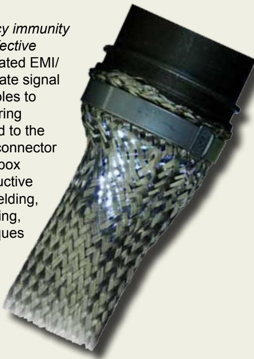
Elimination of apertures or gaps in shields and enclosures is critical, especially for high frequency (short wavelength) EMI. Resolution of low frequency EMI requires thicker shielding material while high frequency EMI is best managed with thin layers of highly conductive material. Use of EMI gaskets, nut-plates, connector ground springs and appropriate types of cable shielding is also critical. AmberStrand® Braid is especially effective since it does not introduce unwanted gaps or apertures.
