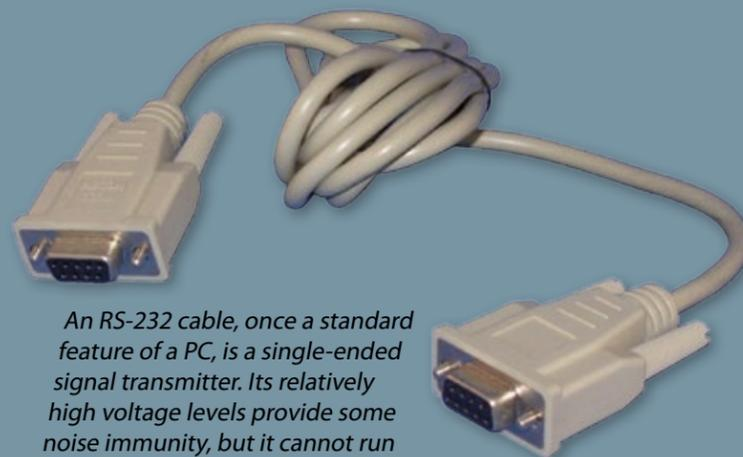
An RS-232 cable, once a standard feature of a PC, is a single-ended signal transmitter. Its relatively high voltage levels provide some noise immunity, but it cannot run at high speed. It has been largely replaced by USB.
