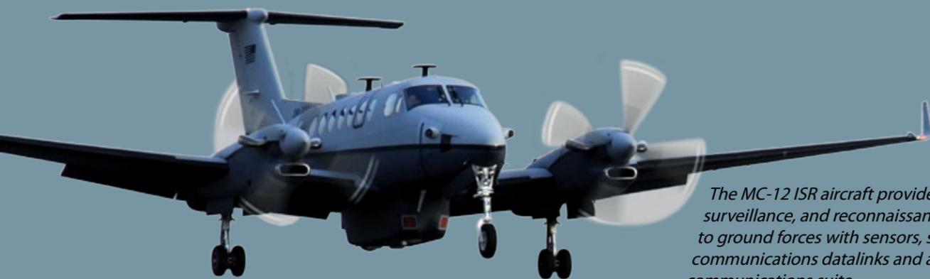
*The MC-12 ISR aircraft provides intelligence, surveillance, and reconnaissance support to ground forces with sensors, satellite communications datalinks and a robust voice communications suite*
