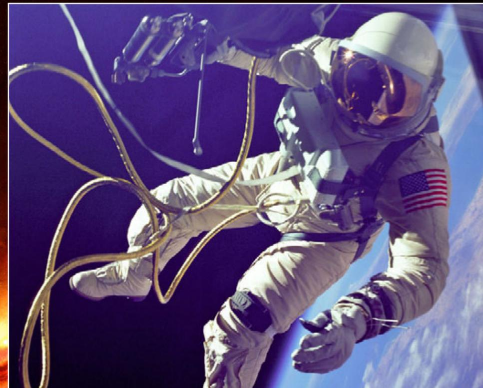
NASA Astronaut Ed White made history on June 3, 1965, when he floated out of the hatch of his Gemini 4 capsule into the void of space for the first American spacewalk. White was attached to the capsule by a 25 foot umbilical cord, Manufactured by Glenair. The golden umbilical was displayed for more than a decade at the Smithsonian National Air and Space Museum in Washington, DC.
