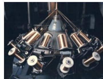
Glenair can also offer ArmorLite™ users direct factory overbraiding services for both point-to-point as well as multi-branch assemblies.
