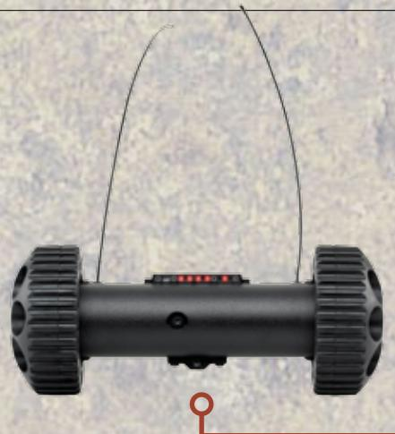
ReconRobotics Recon Scout IR tactical robot designed for tactical and SWAT applications, the man-packable and throwable MUGV is equipped with thermal/IR imaging and video broadcast capability.
