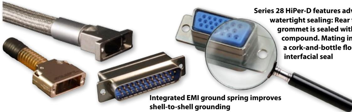
Series 28 HiPer-D features advanced watertight sealing: Rear triple-ripple grommet is sealed with a special compound. Mating interface utilizes a cork-and-bottle flourosilicone interfacial seal
