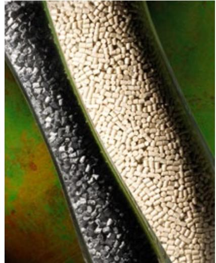
Glenair composite interconnect components are manufactured from 30% glass fiber polyetherimide (PEI), an amorphous thermoplastic with outstanding heat and chemical resistance and high strength.
