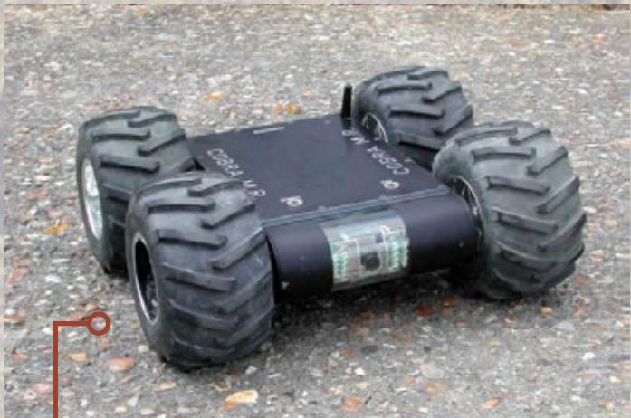
The ECA Inbot is controlled with a PDA or tablet PC and joystick. It is equipped with up to two hours of battery life and a  $\pm 90^\circ$  rotary head with color day/night as well as infrared video.
