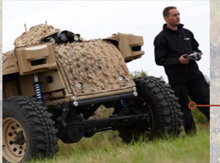
The Mira MACE 2 (Mira Autonomous Control Equipment 2) is designed for load carriage, IED disposal, casualty evacuation and perimeter control. The autonomous controlled vehicle is equipped with a land rover caliber power train and transmission to enhance speed and load-carrying capacity.
