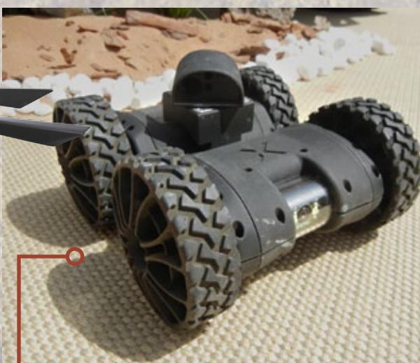
Inspector Bots Toughbot is designed for reconnaissance, security and surveillance. This lightweight UGV features a wide-field video camera, zero turning radius, and an integrated carry handle.
