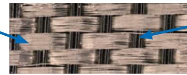
MasterWrap™ is interwoven with high-temperature PEEK composite thermoplastic spring members that ensure up to 95% optical coverage
