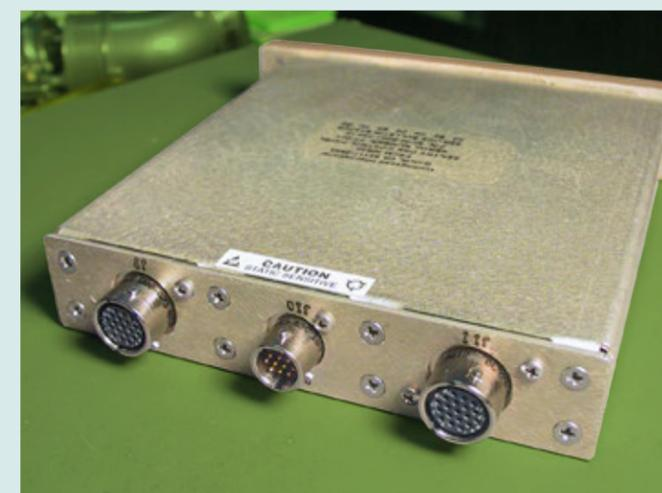
▲ The first Series 803 aircraft application. This cockpit-mounted box controlled the video feed from cabin-mounted cameras.
