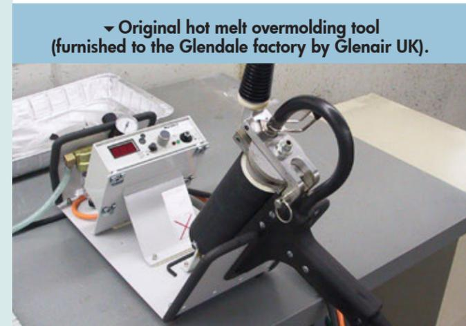
▼ Original hot melt overmolding tool (furnished to the Glendale factory by Glenair UK).
