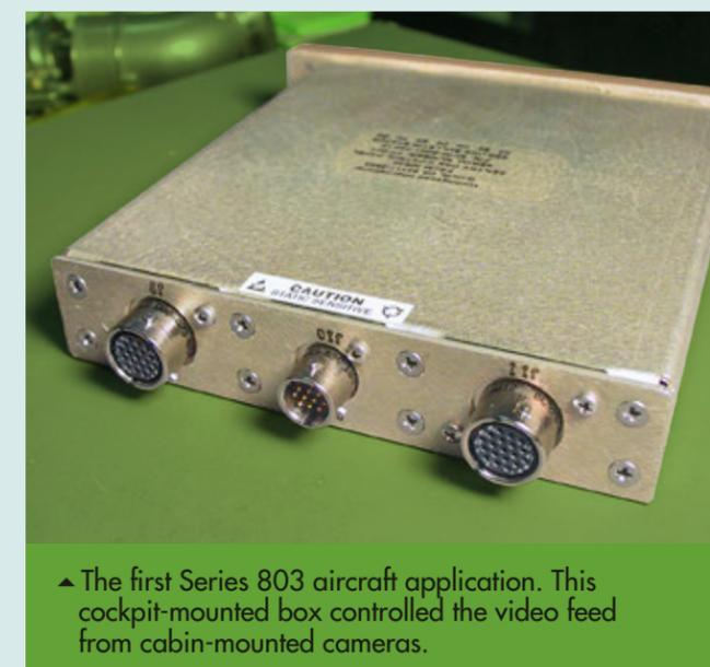
▲ The first Series 803 aircraft application. This cockpit-mounted box controlled the video feed from cabin-mounted cameras.
