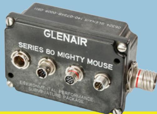
◀ In 2005 we made our first demonstration box. Series 800, 801, 803, and 804 receptacles were mounted into the lid of a composite box. We added a 38999 connector in order to show the dramatic size reduction possible with the Mighty Mouse. Overmolded plugs were supplied with the box, allowing customers to mate and de-mate the four types of connectors.
