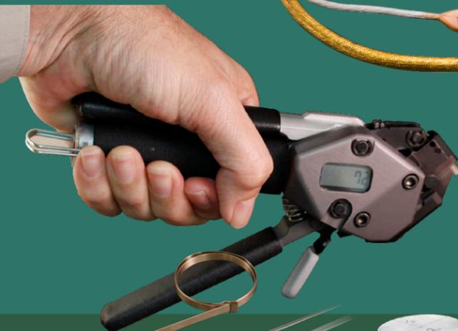
▶ Reliable Band-Master ATS<sup>®</sup> EMI/RFI shield termination technology used extensively throughout the shop
