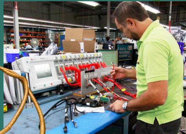
▶ Continuity testing standard on all cable circuits
