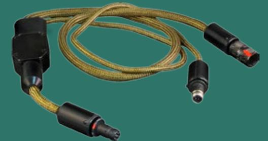
Non-environmental aircraft cable with integrated circuit breakout box and Mighty Mouse 804 push-pull connectors
