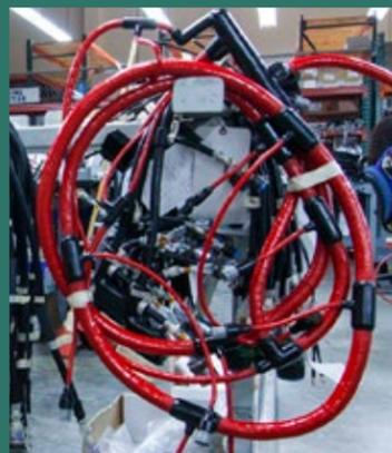
Glenair's hydrostatic test lab accommodates pressure testing of discrete connectors as well as large multibranch assemblies
