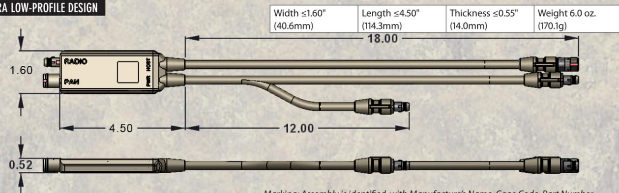
Marking: Assembly is identified with Manufacture's Name, Cage Code, Part Number, Date Code and Serial Number. Dimensions are for reference only.
