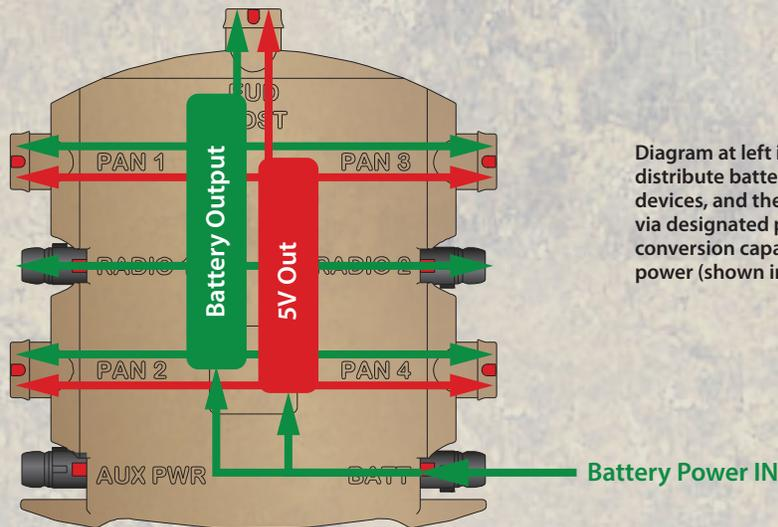
Diagram at left illustrates STAR-PAN's ability to distribute battery power to radios, peripheral devices, and the EUD/host (shown in green) via designated ports. On-board power conversion capability can also deliver 5 Volt power (shown in red) for USB power.
