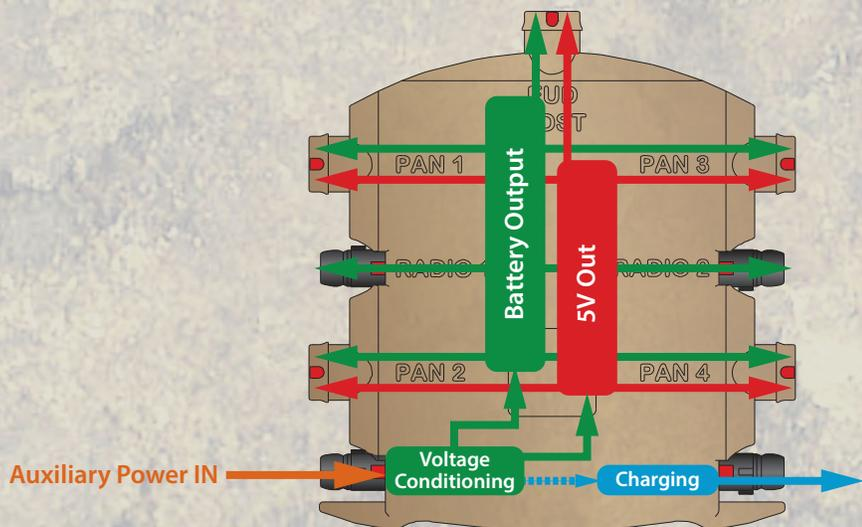
Auxiliary power sources, such as conditioned DC power from vehicles (shown in orange) is conditioned by the STAR-PAN embedded electronic subsystem for use by both standard battery-powered devices (green) as well as compatible 5 Volt equipment (red). The power may be served to both the EUD host port as well as to multiple PAN and radio ports. Finally, STAR-PAN functions as a charging station (shown in blue) to a rechargeable lithium ion smart battery.
