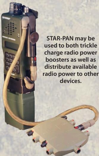
STAR-PAN may be used to both trickle charge radio power boosters as well as distribute available radio power to other devices.
