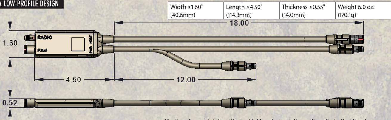
Marking: Assembly is identified with Manufacturer's Name, Cage Code, Part Number, Date Code and Serial Number. Dimensions are for reference only.
