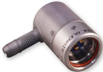
157-008 MIL-DTL-55116 type audio plugs feature 90° cable entry with an integrated, configurable 8-position backshell. 6 conductors accommodation with max Ø .045" insulation each. Available in both 5 pin and 6 pin configurations. Shells are made of passivated stainless steel, contacts are gold plated copper alloy. Plug connector contacts are sealed in the unmated condition.
